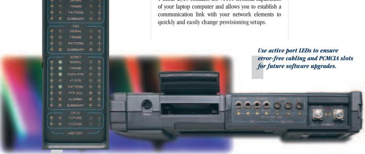
Get immediate feedback of test status with color coded front panel LEDs.
